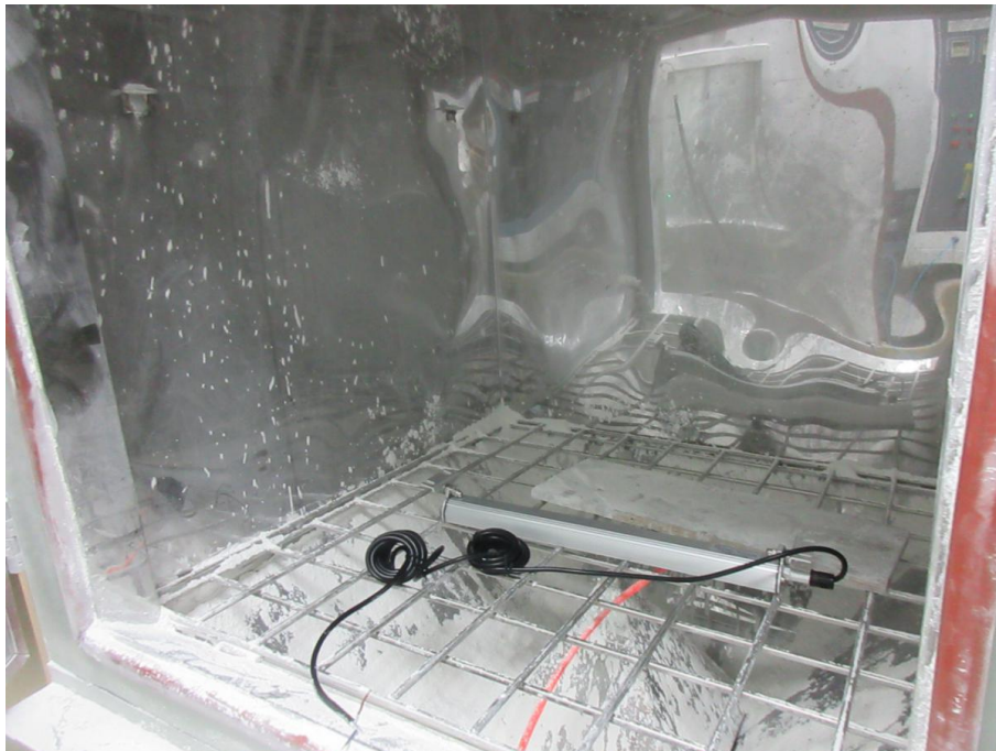
Photo 2: IP6X test of model QLED3-112-1
