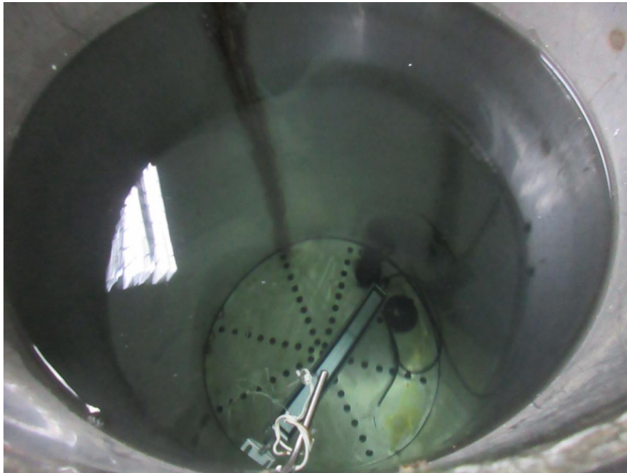
Photo 3: IPX7 test of model QLED3-112-1
